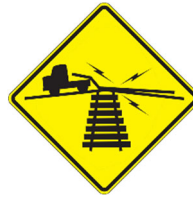
Uneven Grade Crossing
